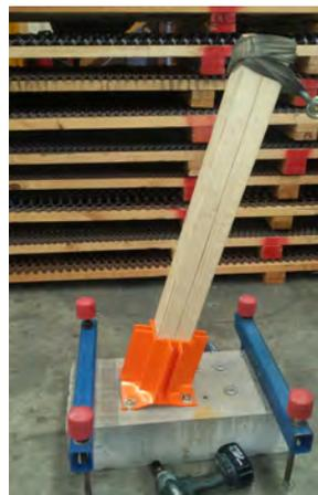
Pic 5 - Safety Base tested to 3160 Newtons without failure
